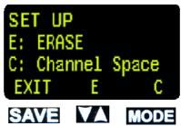
The SET UP-Menu is left with the SAVE key. The device remains switched-on and returns to the normal display mode.
