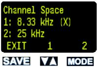
This menu enables to select the desired channel spacing. The actual channel spacing is marked with an "(X)" at the end of the line.
