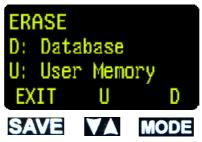
The erasing of the user-defined frequency can now be with the keys. The process takes a few minutes and the display presents the message: "ERASING".
