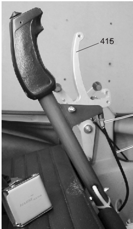
Fig. 3.2/1 Prerotation control cable adjuster
