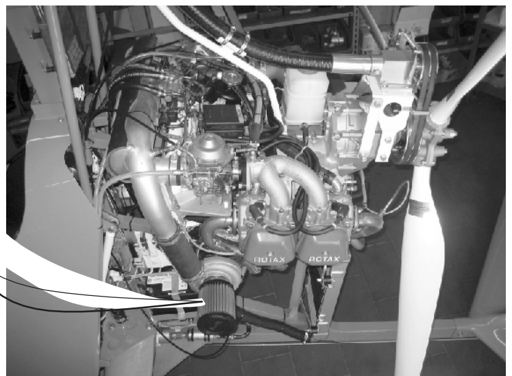
Fig. 3.17/1 Safety wiring for fixation of engine air filter
