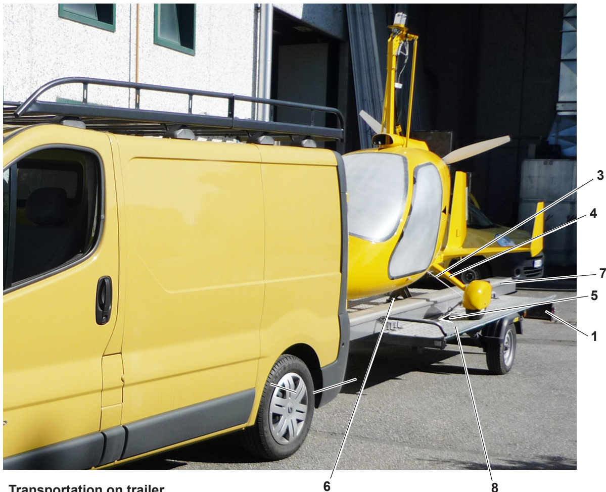
Fig. 6.5/1 Transportation on trailer
