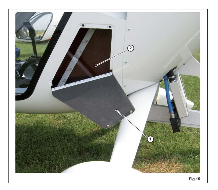
When refuelling it is imperative that the passenger door is fully open. In the event of a fuel spillage on the passenger door window, damage may occur to the transparency. Any fuel spillage on the cowling should be wiped off with a cloth.
