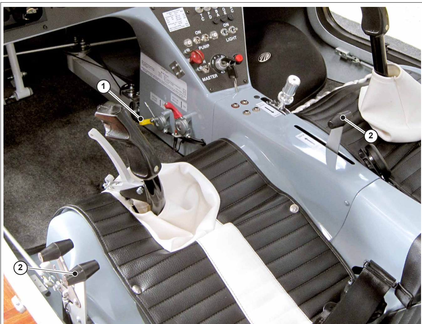
Fig.9 - Choke control lever
