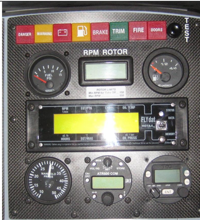
Figure 2 - Central Instrument Panel with New Warning Light Installed
