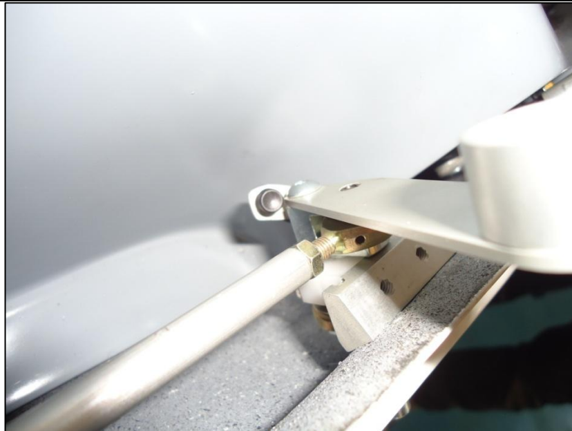
Figure 1 - Correctly Located Detection Switch
