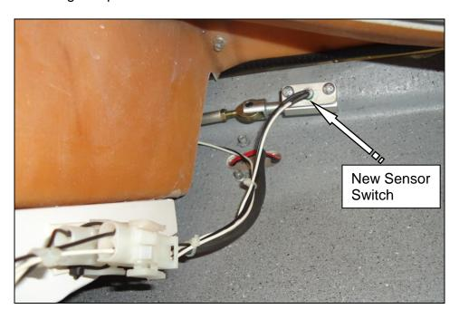
A further switch is mounted on a bracket, located below each of the door locking handles. This switch will only be activated once the handle has been fully pushed into the over-centre 'locked' position.
