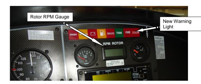
Additionally, if the system registers an incorrectly closed door then the rotor rpm gauge is rendered inactive and will not register a reading until both doors have been correctly latched and locked.
